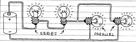
CIRCUITS ARE BOTH SERIES AND PARALLEL. ALL PROVIDE A COMPLETE PATH BETWEEN THE CIRCUIT AND ITS POWER SUPPLY.
