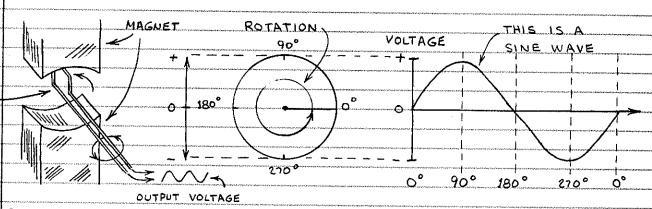
ROTATING COIL VOLTAGE OUTPUT AC SINE WAVE
