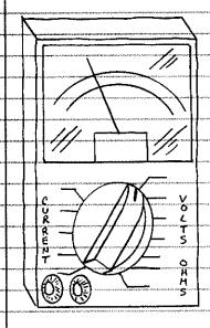
YOU CAN EASILY MEASURE AC AND DC VOLTAGE AND CURRENT WITH AN INSTRUMENT CALLED THE MULTIMETER ANALOG MULTIMETERS USE A MOVING COIL METER. DIGITAL MULTI-METERS HAVE A DIGITAL READOUT. THE MULTIMETER IS THE SINGLE MOST IMPORTANT ELECTRONIC TEST INSTRUMENT.
