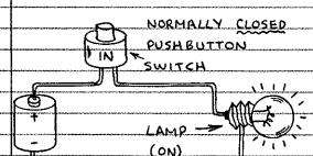
THE LAMP NORMALLY GLOWS. ONLY WHEN THE SWITCH IS OPENED IS THE LAMP OFF. IN OTHER WORDS, THE "NOT" GATE REVERSES (INVERTS) THE USUAL ACTION OF A SWITCH. HERE'S THE TRUTH TABLE:
