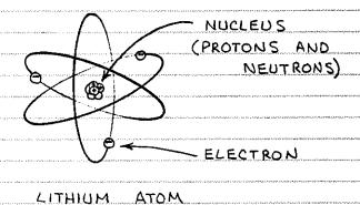
NUCLEUS THIS IS A LITHIUM (PROTONS AND ATOM, THE THIRD SIMPLEST ATOM AFTER HYDROGEN AND HELIUM. LITHIUM ATOMS HAVE 3 ELECTRONS THAT ENCIRCLE A NUCLEUS OF 3 PROTONS AND 4 NEUTRONS.
