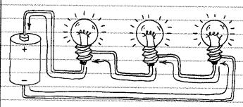
THAN ONE COMPONENT (SWITCH, LAMP, MOTOR, ETC.) A SERIES CIRCUIT IS FORMED WHEN CURRENT FLOWING THROUGH ONE COMPONENT EIRST FLOWS THROUGH ANOTHER. (ARROWS SHOW DIRECTION OF ELECTRON FLOW.)
