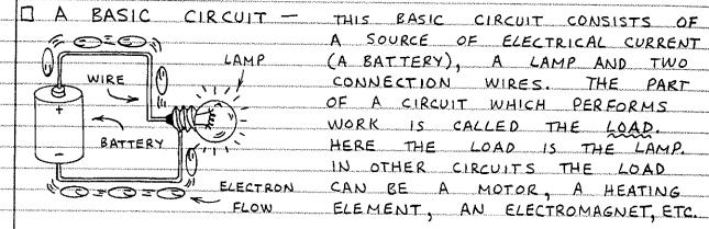
A SOURCE OF ELECTRICAL CURRENT (A BATTERY), A LAMP AND TWO CONNECTION WIRES. THE PART OF A CIRCUIT WHICH PERFORMS WORK IS CALLED THE LOAD. HERE THE LOAD IS THE LAMP. IN OTHER CIRCUITS THE LOAD ELECTRON CAN BE A MOTOR, A HEATING ELEMENT, AN ELECTROMAGNET, ETC.
