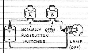
D SWITCH "AND" GATE. THE LAMP GLOWS ONLY WHEN SWITCHES A AND & ARE CLOSED THE TABLE SUMMARIZES THE GATE'S OPERATION, IT'S CALLED A TRUTH TABLE
