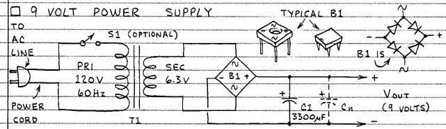
THIS IS A BASIC AC LINE OPERATED 9 VOLT POWER SUPPLY.
