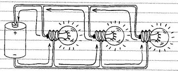
WHEN TWO OR MORE COMPONENTS ARE CON-NECTED SO CURRENT CAN FLOW THROUGH ONE COMPONENT WITH-OUT HAVING FIRST TO ELOW THROUGH ANOTHER.
