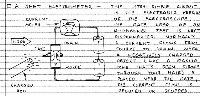
IS THE ELECTRONIC VERSION OF THE ELECTROSCOPE. THE GATE LEAD OF AN N-CHANNEL JEET IS LEFT DISCONNECTED. NOR MALLY A CURRENT FLOWS FROM SOURCE TO DRAIN, WHEN A NEGATIVELY CHARGED OBJECT (LIKE A PLASTIC COME THAT'S BEEN STROKED THROUGH YOUR HAIR) IS PLACED NEAR THE GATE. THE CURRENT FLOW IS REDUCED OR STOPPED.
