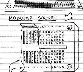
CUTAWAY SHOWING COMMON TERMINAL CONNECTIONS.
